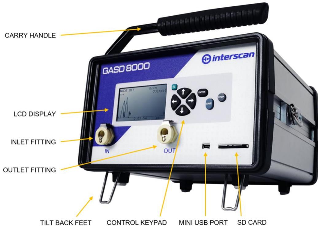
**LCD DISPLAY** – Displays all relevant numeric and text information related to sampling and menu navigation. Gas values can be displayed numerically or graphically. See section **3.1.1 – Display Fields And Indicators** for display details.
