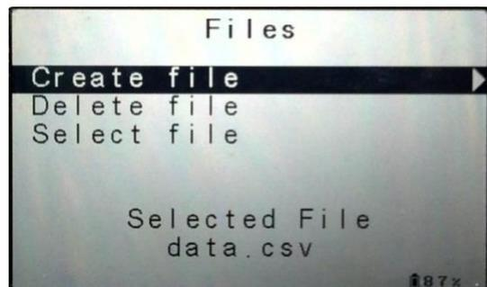
**Create file** – Shown on the right. Use the **RIGHT ARROW** button to highlight the name field then use the **UP/DOWN** arrow buttons to change the character as desired and the **RIGHT/LEFT** arrow buttons to move the character position as desired. Press the **SAVE** button when finished to save the new file.
