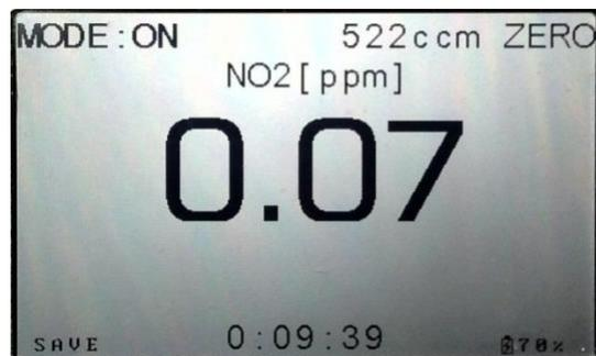
When finished with sampling, press the **STOP BUTTON** once from ON MODE to return to OFF mode. This stops the automatic data storage saving data space and battery life.
