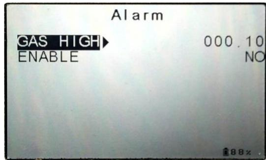
Highlight this parameter then use the **RIGHT ARROW** button to highlight the numeric field(s) you wish to change. Use the **UP** or **DOWN ARROW** buttons to change the numeric value of the desired fields. Once satisfied with the value, use the **LEFT ARROW** button to exit the parameter value field.
