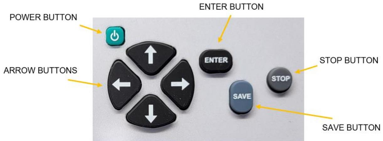
**POWER BUTTON** – Press to turn power to instrument ON. Press from the MAIN MENU to turn power OFF.
