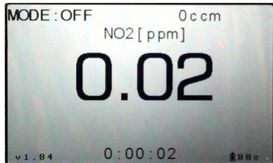
This is the mode the instrument should be kept in when powered but not in use. To advance to ON MODE from OFF MODE, press the **ENTER** button. To return to the main menu from OFF MODE, press the **STOP** button.
